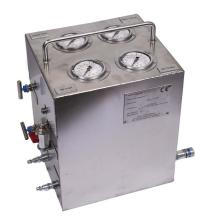
Unique to our cutting solutions is our water control box, designed to regulate the flow of air and water. Its purpose is to control whether the tool is permitted to start or not
